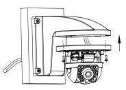
(6) Install the housing and lock the screws.
