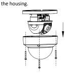
6 Loosen the tightening screw and take down
