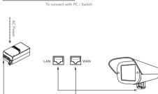
To connect with IP Camera (PoE can be enabled for LAN)
